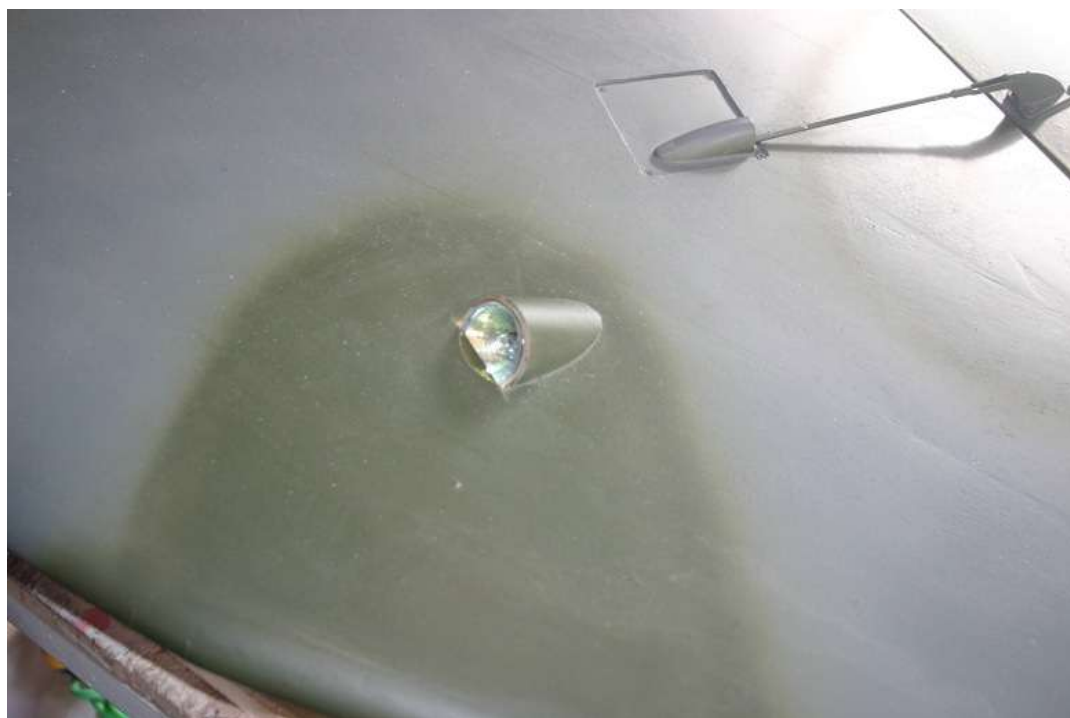
10 watt Halogen landing light
