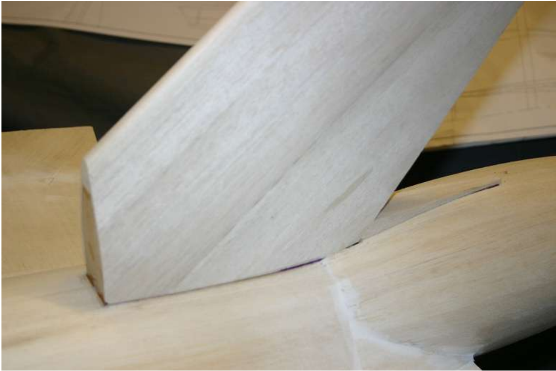
Cut opening in turtle deck against F14 but don't cut through 6mm sq longeron
