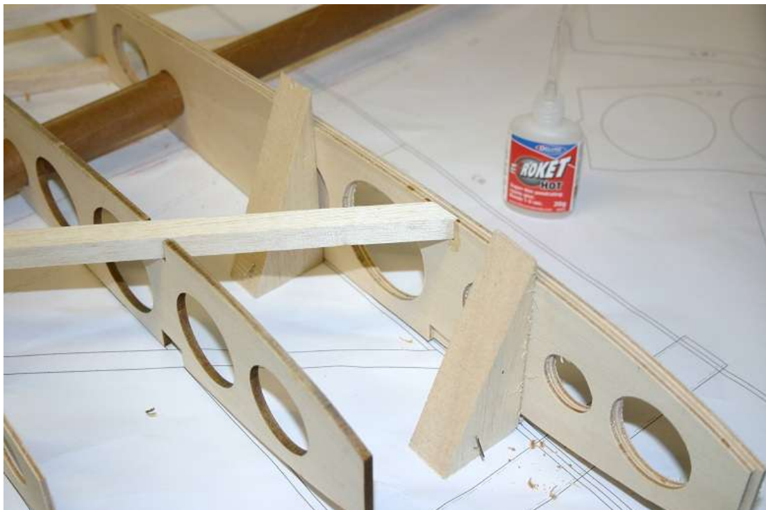
Use right-angle blocks to keep W4 & W5 square
