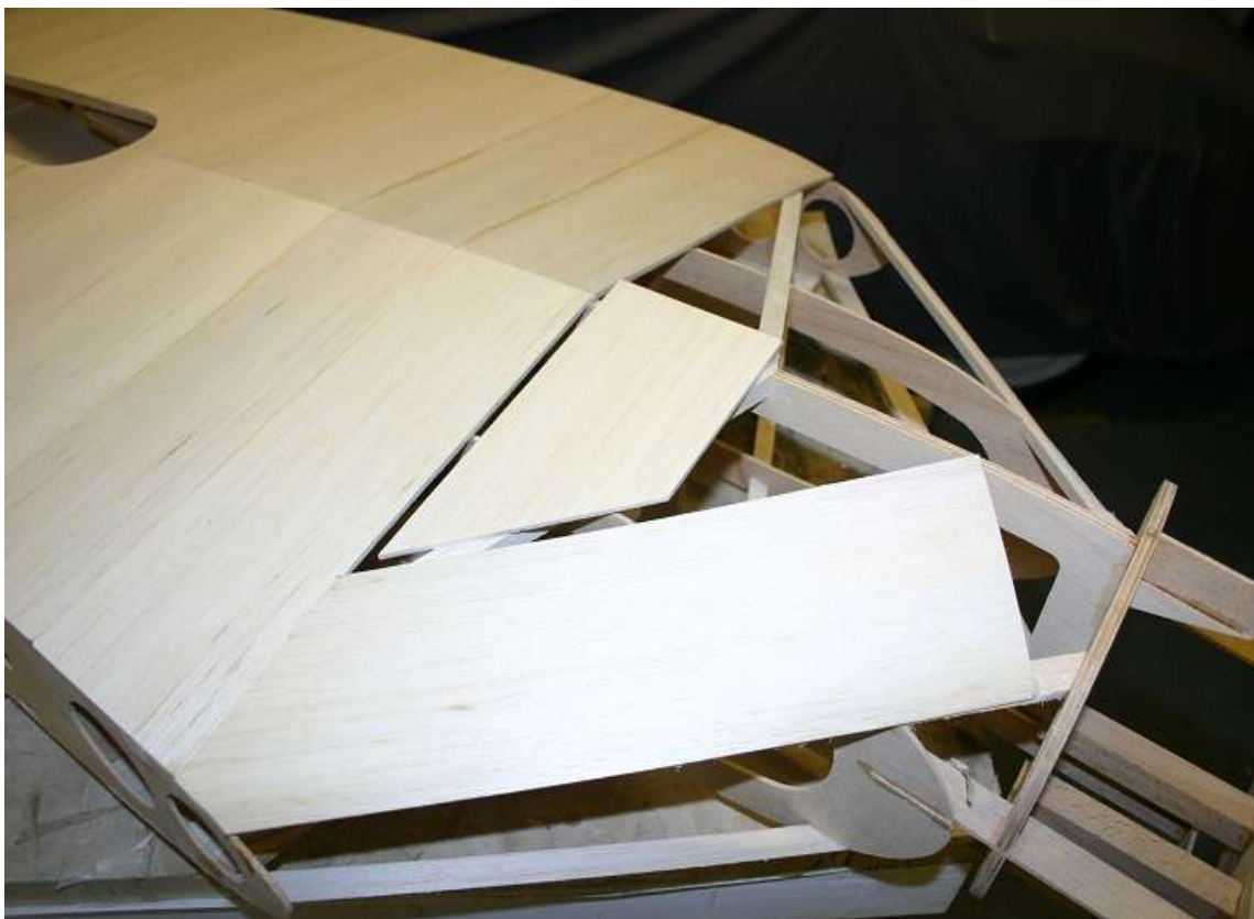
Continue to sheet top of fuselage noting grain direction
