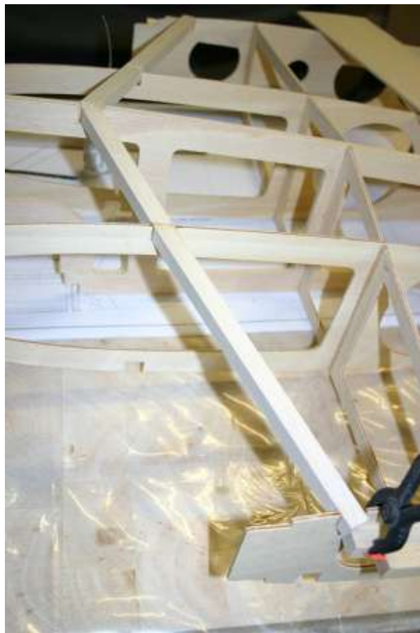
Add front spar. Note; spar to be cut notched at W2
