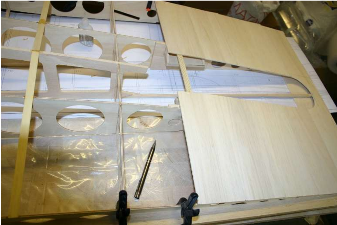
Add top sheeting in sections. Note importance to keep W3 straight
