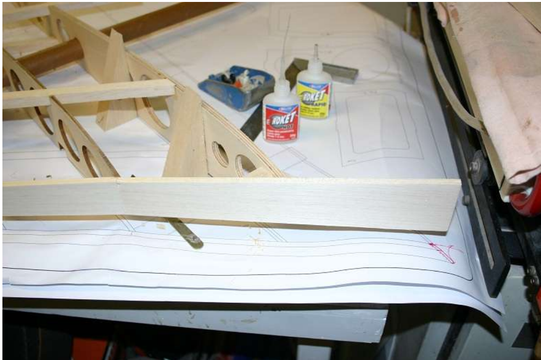
Fit 'inner' part of inner leading edge 'THIRD'
