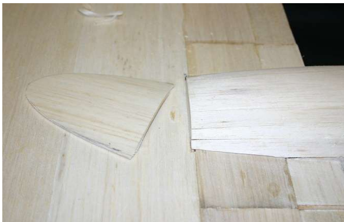
Under fairing from solid balsa
