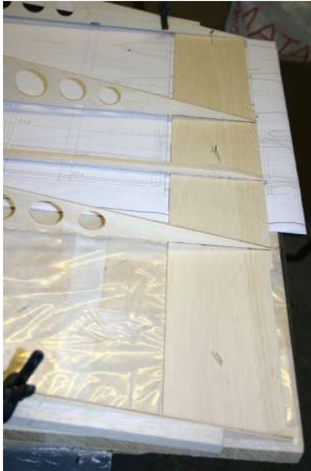
W1, W2 & W3 all lined up flush with sheet edge
