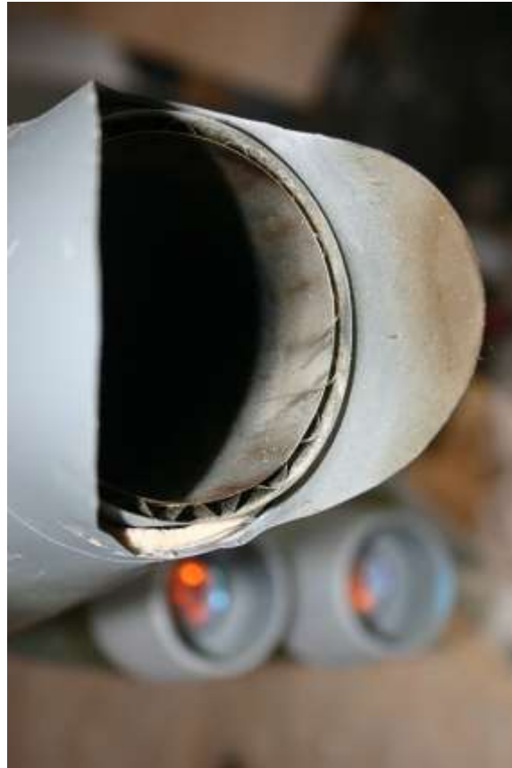
Tail pipe crown designed to give 'dome' appearance from a side view
