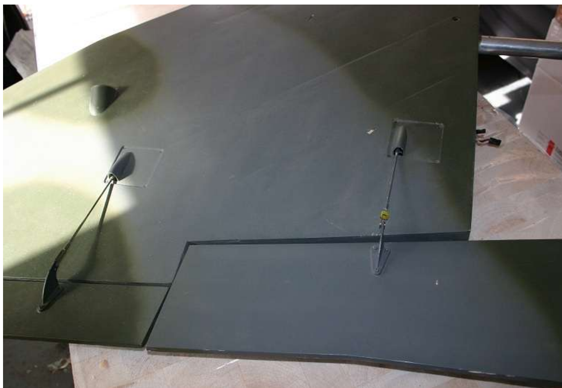
Out servo operates in elevon mode and inner servo as elevator only
