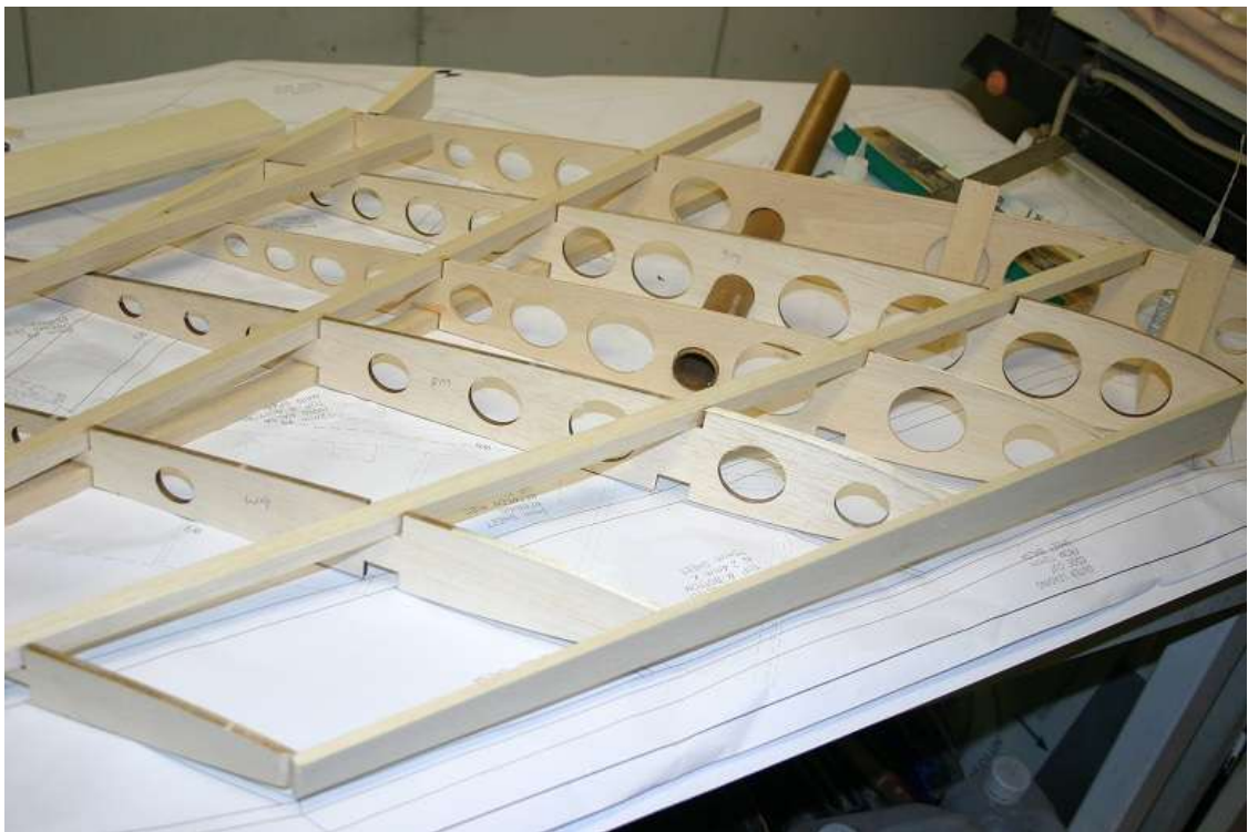
Fit 'middle' part of inner leading edge 'FIRST'
