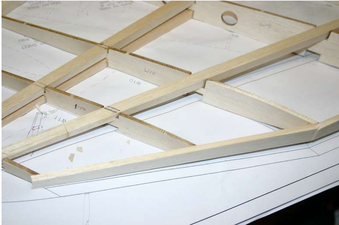
Fit 'outer' part of inner leading edge 'SECOND'
