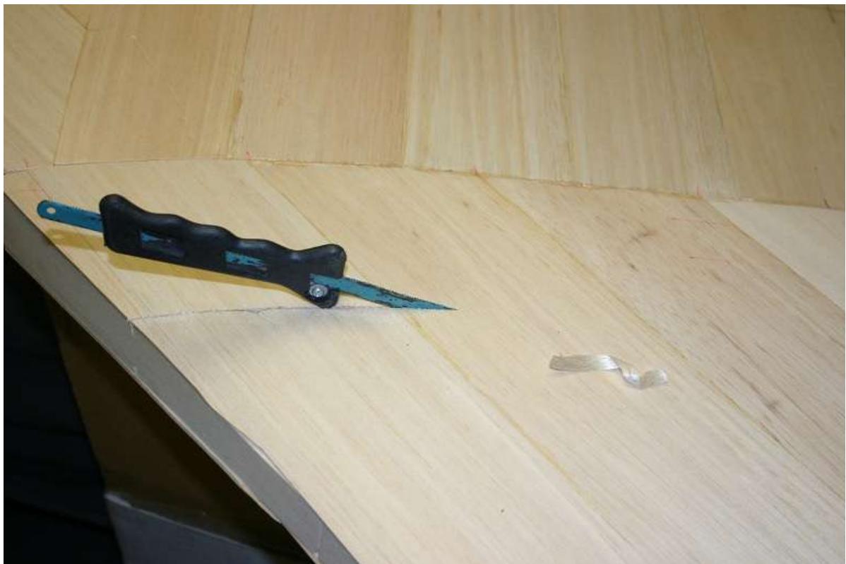
Part the wing from the fuselage by cutting between W4 & W5 with a hand saw
