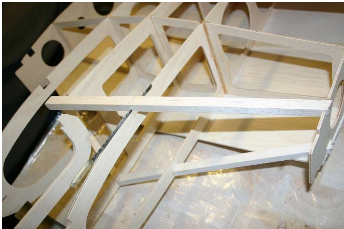
Add forward bottom spar. Note; spar cut notched at W2
