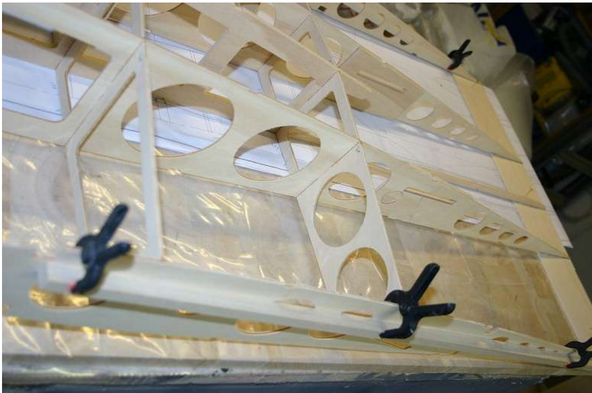
Add FS3, FS4 and W3 and glue to end sheet. Note; use wing spar and clamps to keep W3 straight and true
