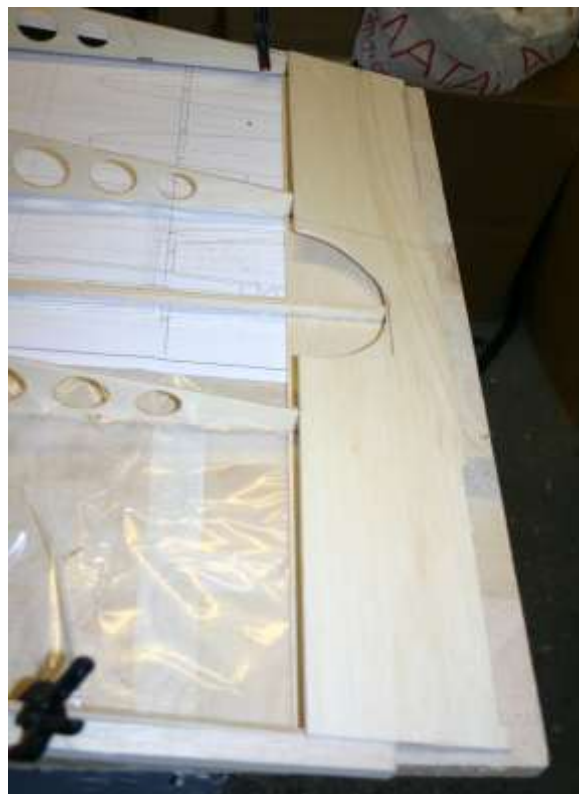
Start to top sheet from rear noting scalloped section to allow thrust tube the pass
