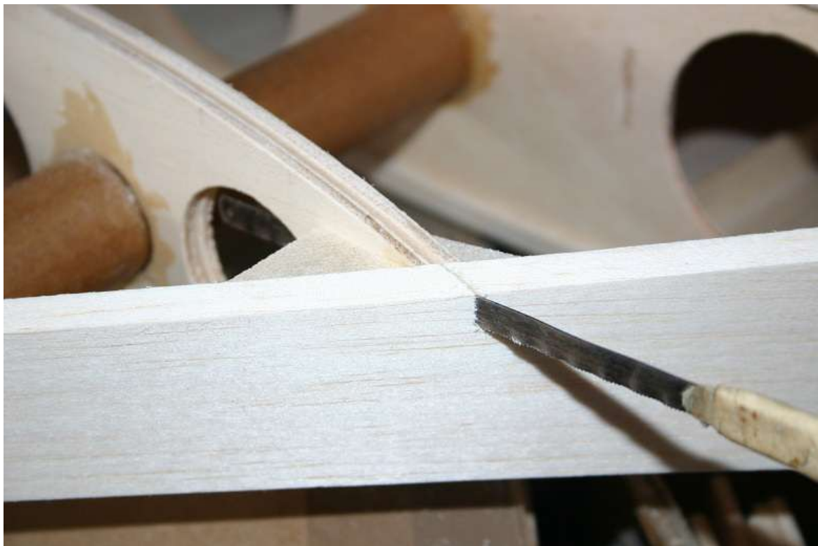
Chamfer leading and trailing edges flush with wing ribs. Make a small cut in the leading edge between W4 & W5 as a location point to part the wings from
