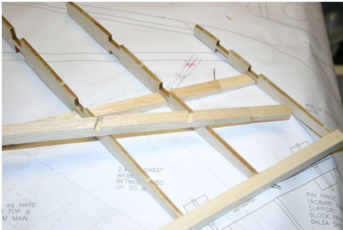
Chamfer and notch top rear spar similar to bottom
