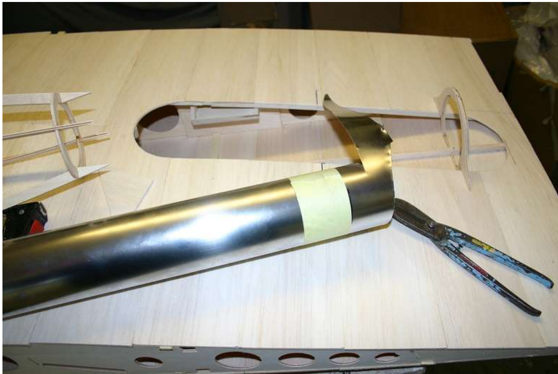
Standard 600mm long thrust tube (from WREN Turbines) trimmed to length
