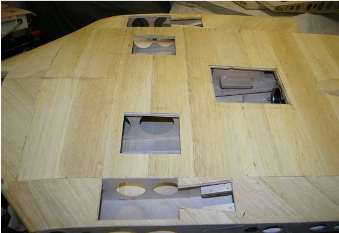
Indication of hatches required in the underside. Model is finished in glass cloth epoxy
